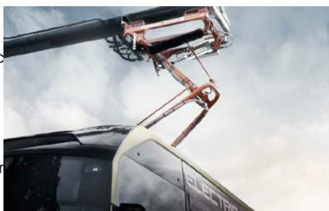
Figure 3 Detail of charging fixture and pantograph
