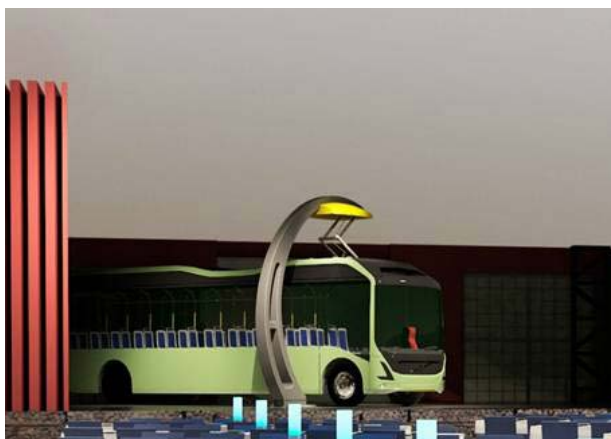
Figure 1 ElectriCity Electric Bus with charging fixture
