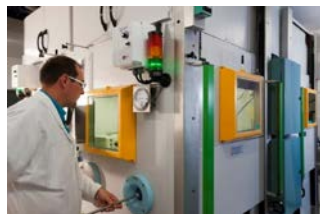
Lead-shielded hot-cell Source CEA LDM-TEP
