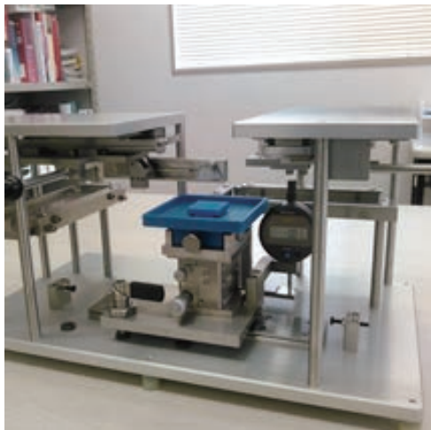
Fig.8: "3D biomaterial micro cutter" an instrument to cut biomaterials into micro size dices Shibata System Service Co., Ltd.: http://www.shibata-sss.com/htm/hightech/en_product.htm
